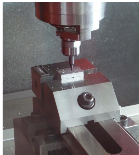
Figure 1. Experimental setup for micromilling of channels in ultrafine-grained metals.
